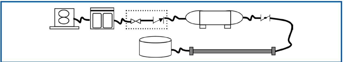
When access is restricted at the exit of the piping, a vessel rupture blow can be performed. Air is compressed in the vessel and then rapidly released by the valve.
