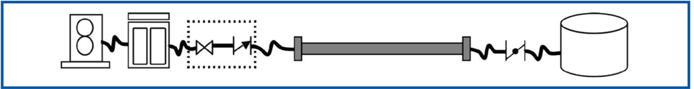
In a standard rupture blow configuration, the piping to be cleaned is pressurized with an air compressor and dryer until it reaches the engineered pressure. Once there is sufficient pressure in the line, the air is quickly released from one end of the piping. The rapid depressurization of the piping blows any loose debris out of the pipe.
