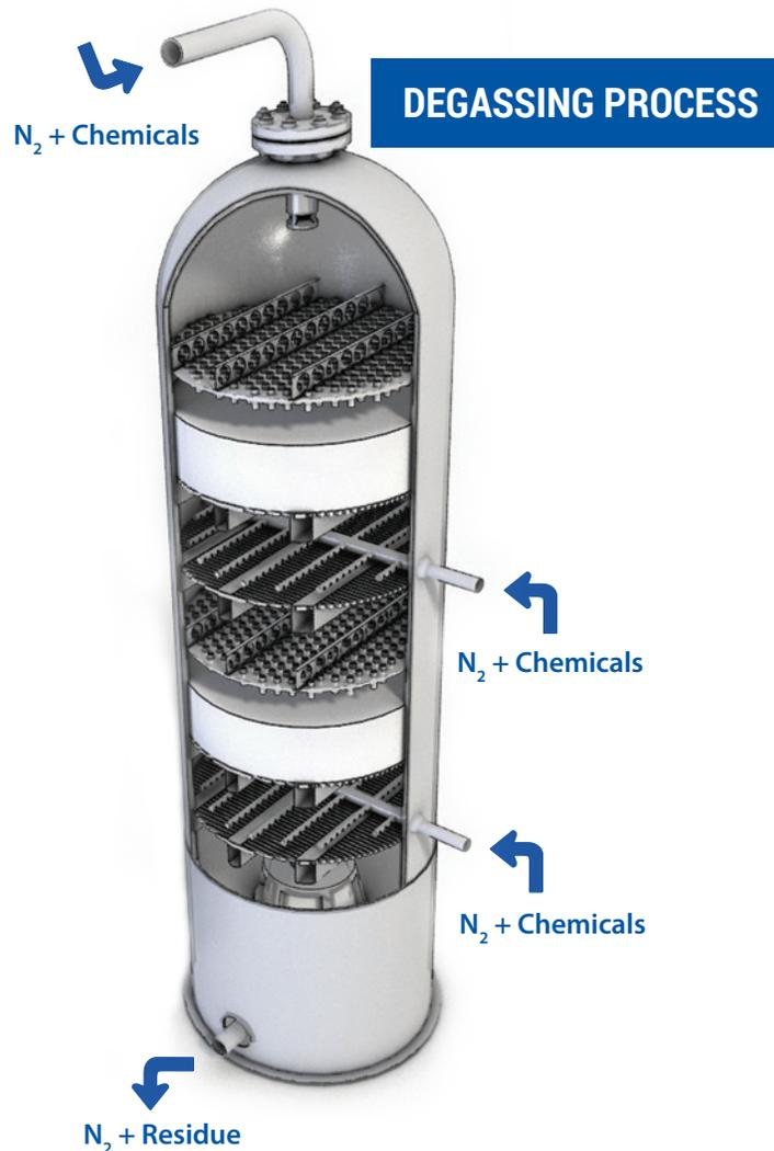
*Inlet and outlet points on reactor vessel*
